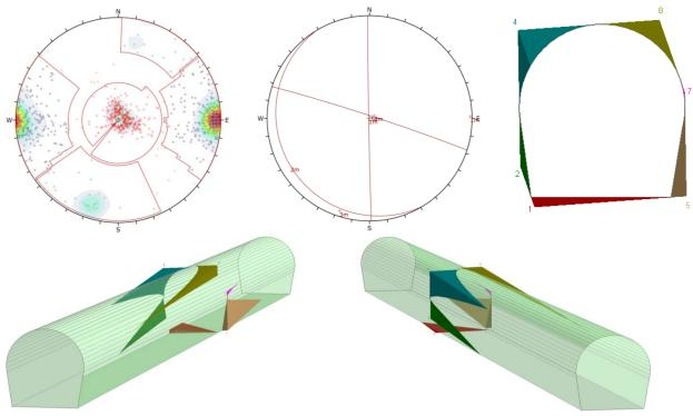
Joint sets and wedges (blocks) formed in an ideal tunnel profile. 160-200m (max localized bolt loading = 0.75 tonnes/m<sup>2</sup> of face area.)
