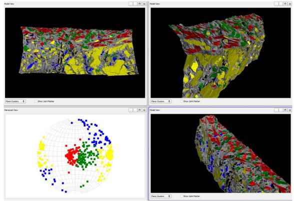
Example of mapping process using lidar scanning. (planes are identified as indicated by colours).
