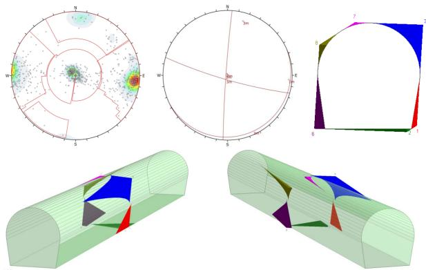
Joint sets and wedges (blocks) formed in an ideal tunnel profile.200-240m (max localized bolt loading = 0.85 tonnes/m<sup>2</sup> of face area.)
