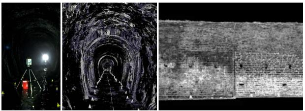
Example lidar intensity images. Left: Lidar survey instrument; (mid) inside view of rock-brick interface; Right: transition between styles of brick work in walls and in the roof.
